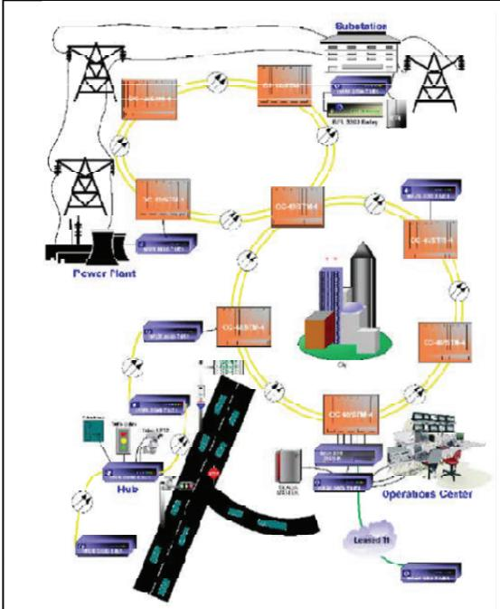
Above is an example of a typical utility / traffic system solution. It is made up of two SONET/SDH rings as the communications backbone. The UCC 2020 T1/E1 Multiplexers are configured to work in a Point-to-Point, Star and Stand-Alone Linear topology over the SONET/SDH system.
